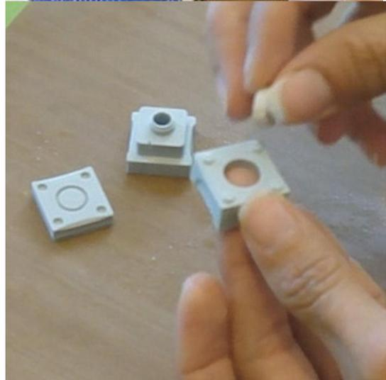
6. Place top layer on the middle layer .Turn upside down and neatly push clay so it evenly fills middle layer shape cavity
