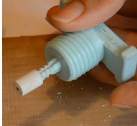
2. Use part assembled part 6A & 6B to slowly screw male part into. Once again open and clean clay dust out frequently.
