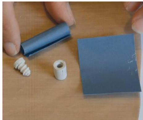
2. Insert this rolled sandpaper in female part and spin part to sand
