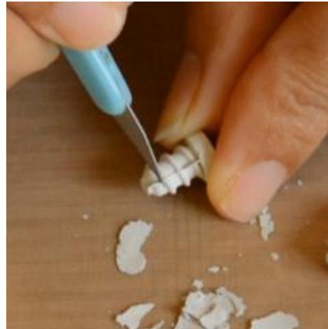
22. Using female part carve opening wider at slight angle. This will make engaging threads easier.
